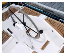
Optional transom lockers close the aft end of the cockpit off and add to the ample stowage
