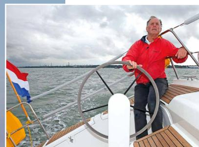
With the wheel canted to windward, the helm is snug in the pushpit and the telltales are visible
